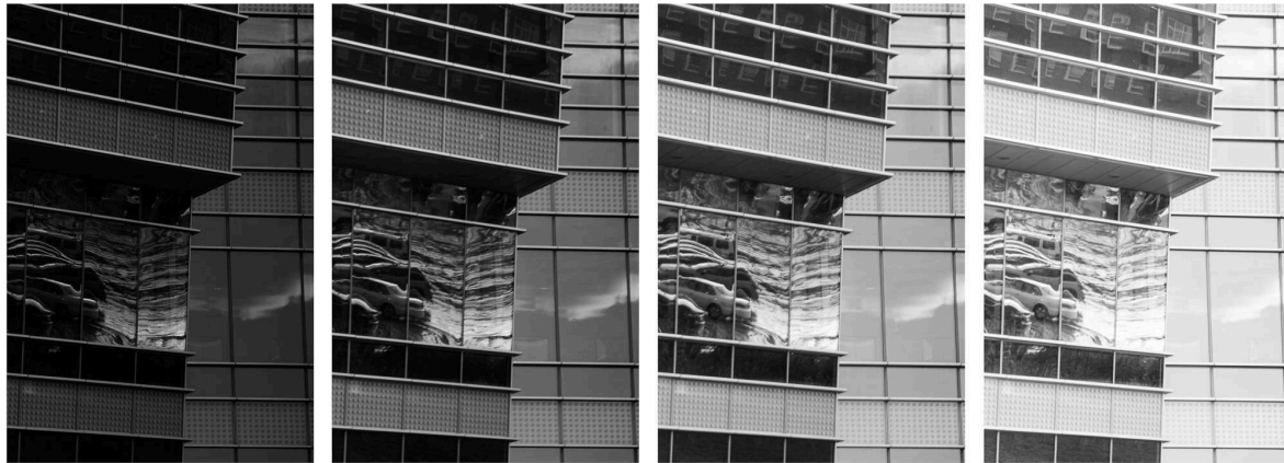
Fig. 6: Difference in image brightness with changing exposure times. Short times correspond to darker images, long times to brighter images.
