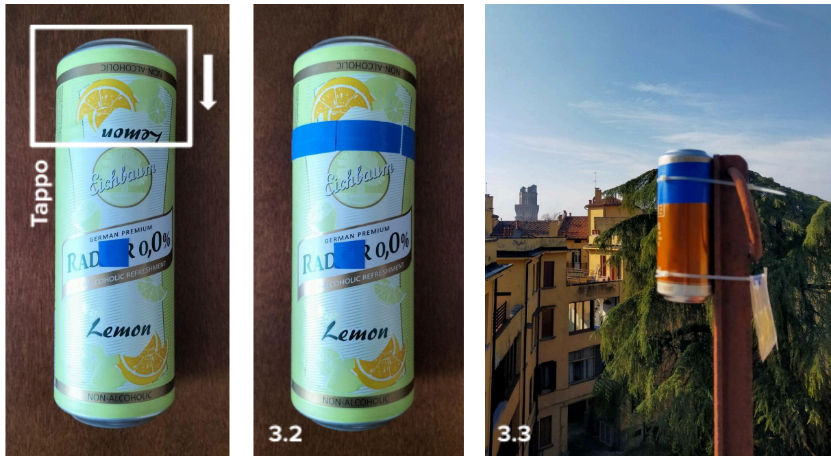
Fig. 3: Closure, sealing, and external positioning of the solar can. The piece of tape above the hole should be removed once the can is fixed to the support.
